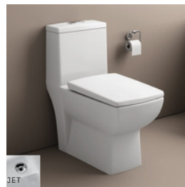
LIBIA One Piece Closet With Jet / Without Jet 715 x 385 x 760mm S Trap Dist. 225mm P Trap Dist. 180mm
