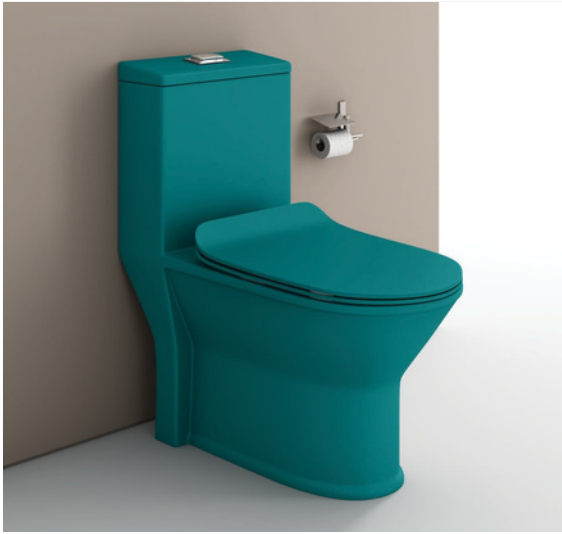
OPAL Rimless One Piece Closet, Siphonic / Washdown Flushing MATT AQUA GREEN 715 x 380 x 775mm S Trap Dist. 100, 225 & 300mm, P Trap Dist. 180mm
