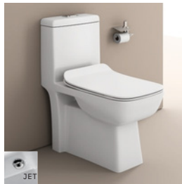
BEETLE One Piece Closet with Jet / without Jet 655 x 350 x 740mm S Trap Dist. 100 & 225mm P Trap Dist. 180mm
